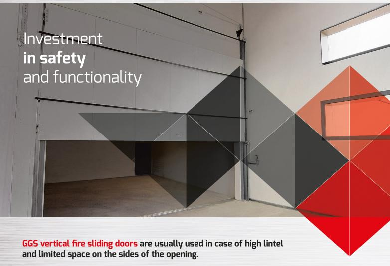
Door closing is typically gravity-operated or using one of the offered motors. The door may be supplied with an emergency exit door with or without a threshold, and equipped according to individual needs. Doors are available in a smoke control or an Ex version.
